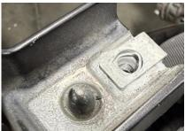
✓ You will need to remove the crash bar and sensors, before you install the center section of your intake to accommodate the larger center section. When reinstalling the crash bar, it must be rotated 180 degrees and the sensors reinstalled on the opposite side. You will also need to drill a new guide hole large enough to align with the guide pin as shown. A step drill bit can be used.
